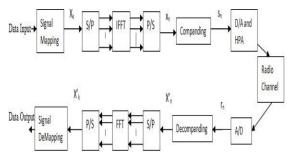
Figure 1: Block Diagram of OFDM System with Companding Technique In the  $\mu$  law companding, compressor squeezes the signal at the transmitter site according to the following formula:
