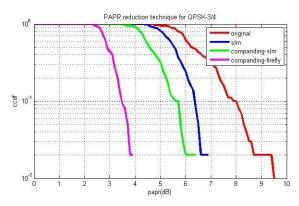
Figure 3. Distribution of PAPR for different PAPR reduction schemes for QPSK
